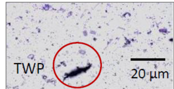
Tire wear particle sampled in the Dreisam (Greifenegg Brücke); photo: Judith Johannsen
